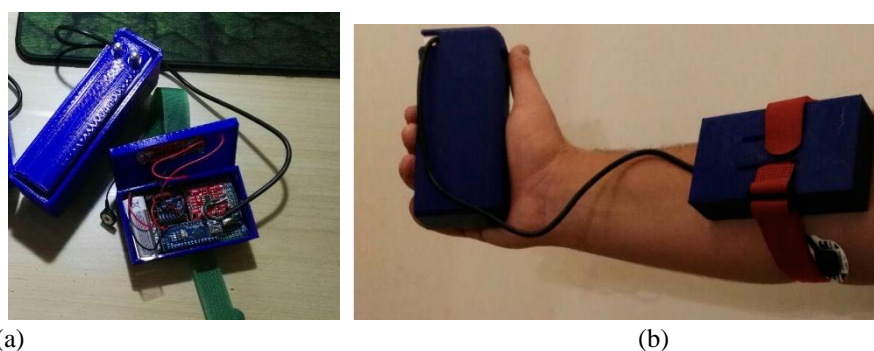
Fig. 3. (a) The proposed prototypal wearable device; (b) the realized device worn by a patient.
